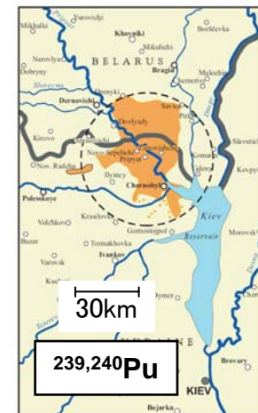
FIG. 3.9. Areas (orange) where the surface ground deposition of ^{239,240}\text{Pu} exceeds 3.7 \text{ kBq m}^{-2} [3.4].
